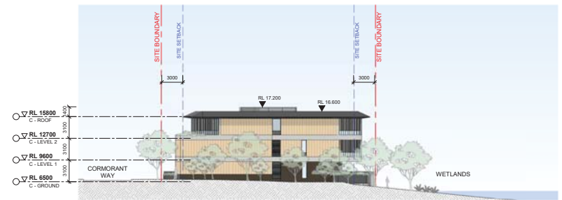
2 BUILDING C - WEST ELEVATION
